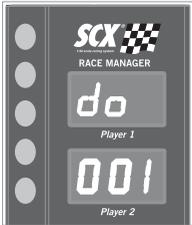
By pressing button A button (repeatedly) we increase the laps, 1 by 1, or (keeping the button pressed) 10 by 10. To confirm the number of laps you have to press button B. To start the race press button B again. The race starts once the five LED lights have gone out, lighting up consecutively, each one accompanied by a beep.
