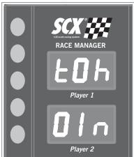
Using button A select the time that you want, (by pressing consecutively) increasing the minutes 1 by 1, or (by keeping the button pressed down) 10 by 10.
